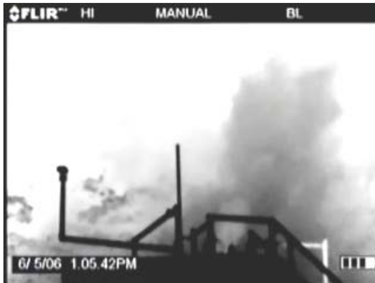
Figure 3. Condensate tanks, which store volatile liquid petroleum produced with natural gas, can be a significant source of VOCs. Emissions are invisible to the naked eye, but can be observed with the use of infrared technology. The picture above is a condensate tank in Weld County, Colorado. Below is the same tank with VOC emissions visible through an infrared camera (images from video prepared by the U.S. Environmental Protection Agency).
